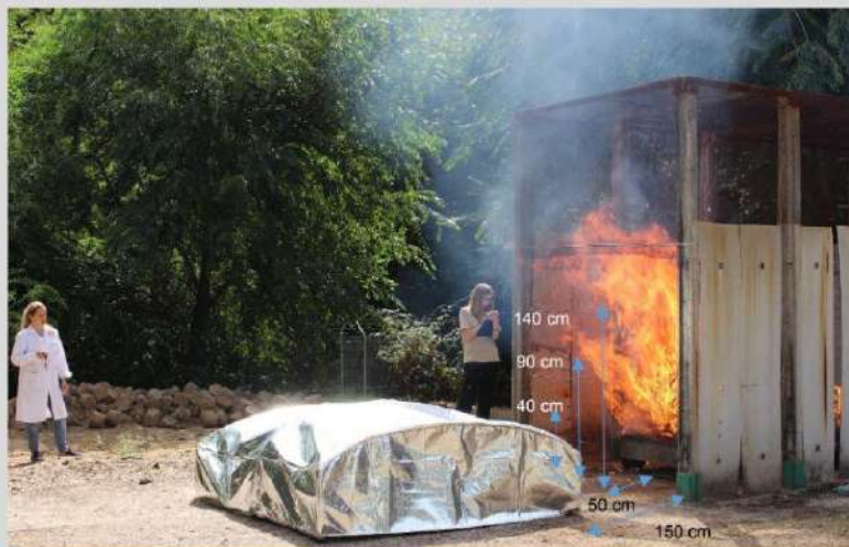
Direct flame contact test INIA (MADRID)
