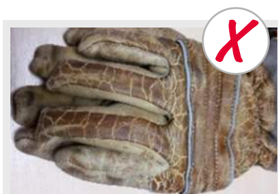
Washing and fire damage
